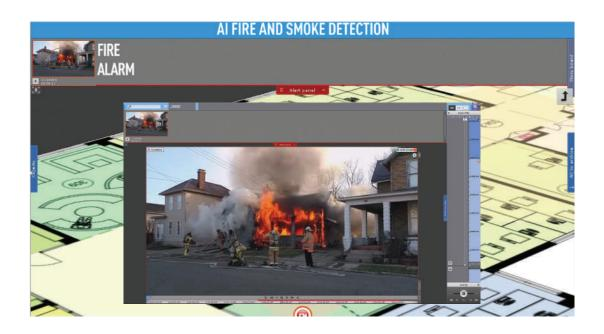
Intelligent video detection of flames and smoke, based on artificial neural networks, works where other sensors are useless. It provides early visual fire detection and a significant reduction in the risk of fire damage.
