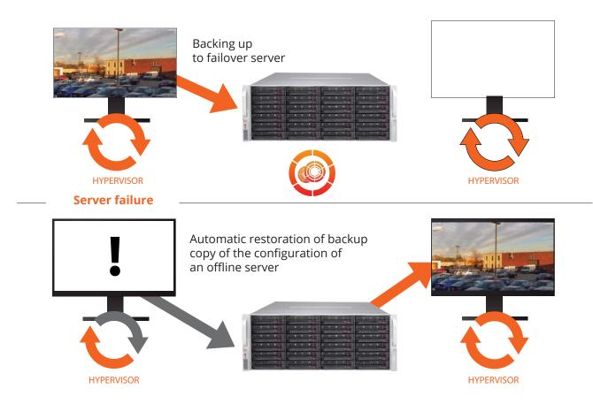
A server can be selected during system configuration to act as a hot standby in case of failure of a main server. The failover server automatically steps in, performing all the functions previously handled by the hardware that is temporarily off-line or malfunctioning. A special hypervisor service monitors the health of all servers in a domain.
