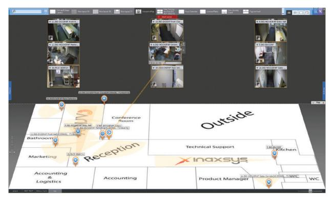
**The interactive 3D map** is a set of ordinary raster blueprints for a site, placed on the screen under viewing tiles, which are displayed in a lifelike projection. On the map you can indicate the location of the cameras included in the layout, as well as mark sensors and detectors. Click a viewing tile to immediately see where the relevant camera is located on the map.
