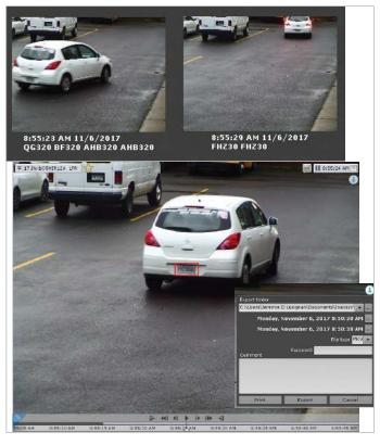
Arkiv features a face and LPR search algorithm that automatically detects a face or a license plate in the field of view or in a provided video footage of one or several cameras.
