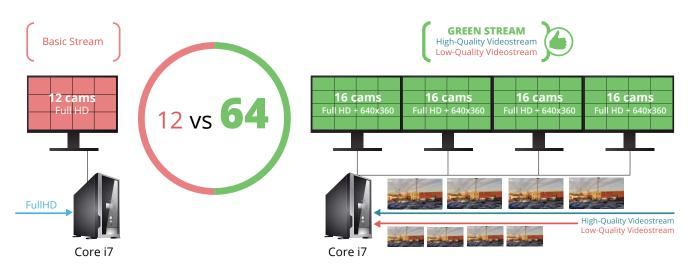
The GreenStream feature automatically chooses a video stream from a camera to the server, and then to the client, depending on the resolution at which the video is currently displayed on the client.
